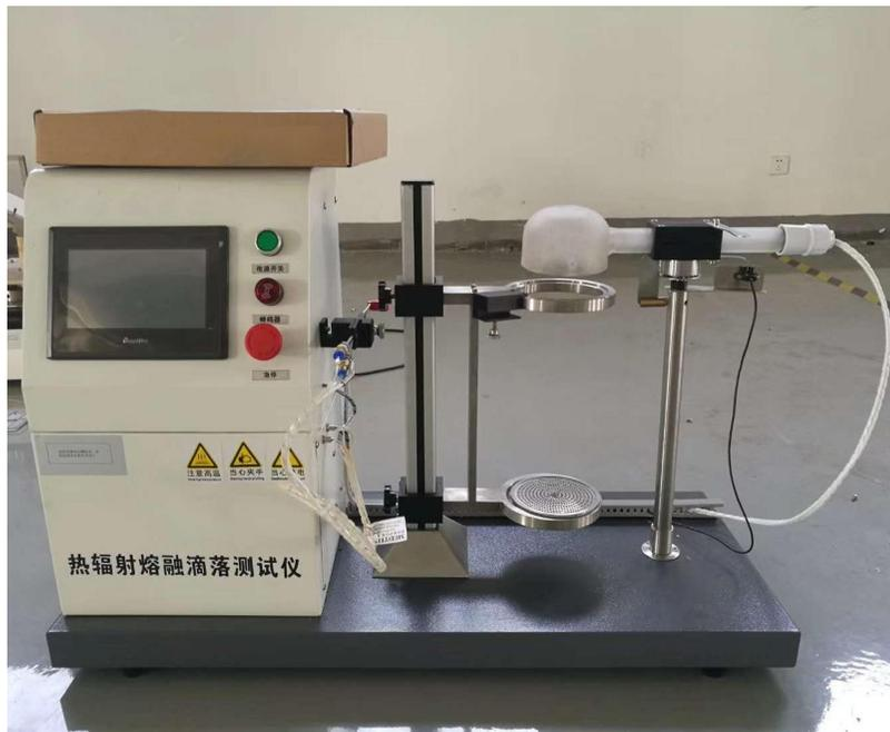
This instrument meets international standards NF P92-505, EU 95/28/EC, ECE technical specifications and requirements of R118 Annex 7 of these Regulations. According to NF P 92-505 request, the test is additional for M-class building materials. It is suitable for hot melt material effect in the primary heat source to evaluate the performance of dripping and burning performance testing. Flexible and thin materials can also be tested.
